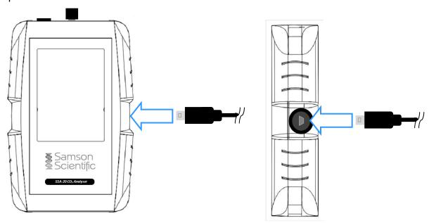
IMPORTANT NOTE: Connecting the charger improperly may cause serious damage to the device. Any damage caused by misuse is not covered by the warranty.
