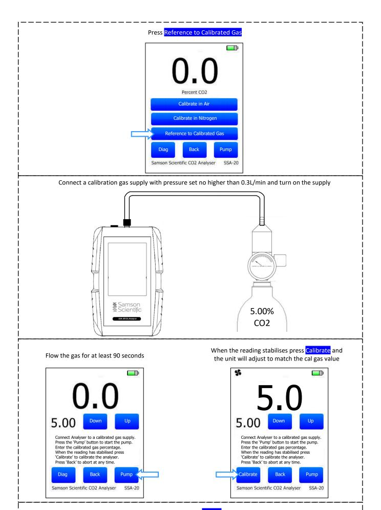
Turn off the gas supply and press the Pump button to switch off the pump.
